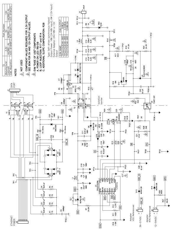
Figure 1. TPS23753EVM-004 Schematic
