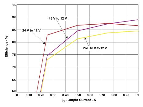
Figure 5. TPS23753EVM-005 Efficiency With 12-V Output
