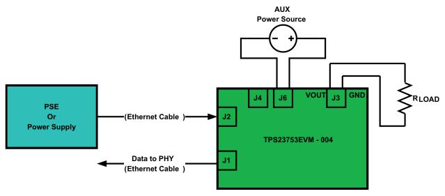
Figure 2. Typical TPS23753EVM-004 Test Setup
