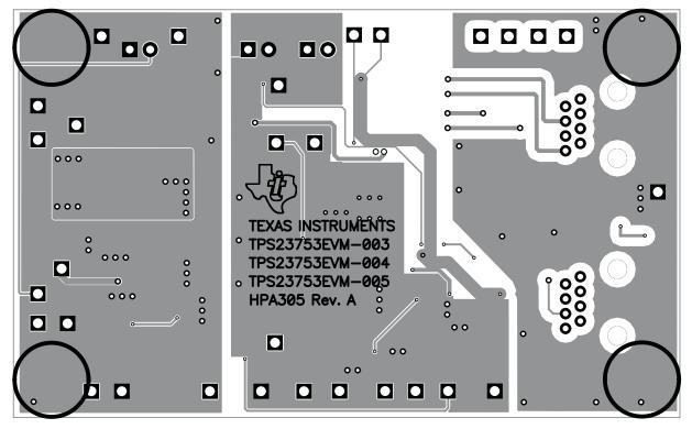
Figure 8. Bottom-Side Routing
