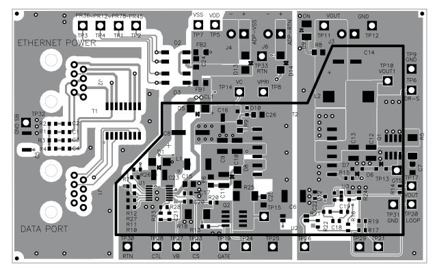
Figure 7. Top-Side Routing
