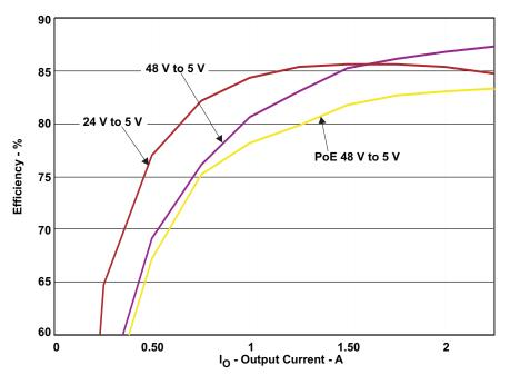
Figure 4. TPS23753EVM-003 Efficiency With 5-V Output
