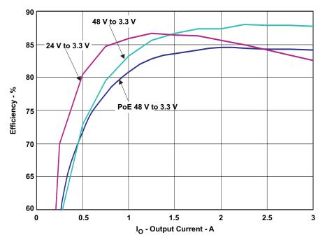
Figure 3. TPS23753EVM-004 Efficiency With 3.3-V Output
